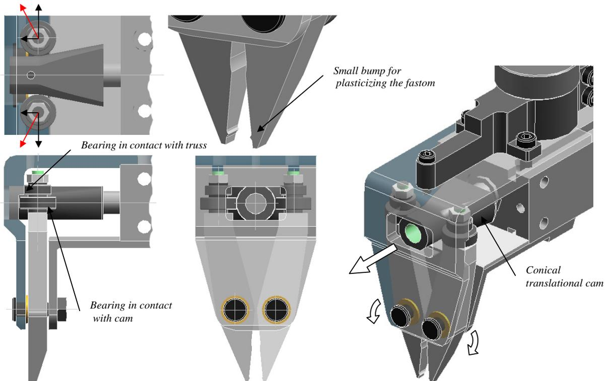
Fig.4: The pneumatic plier for wire crimping. It also acts as a truss for the multifunctional end-effector.
