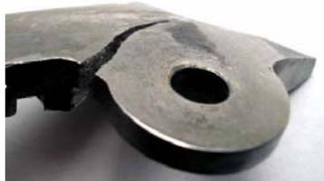
Fig.5: Structural failure of old pliers
