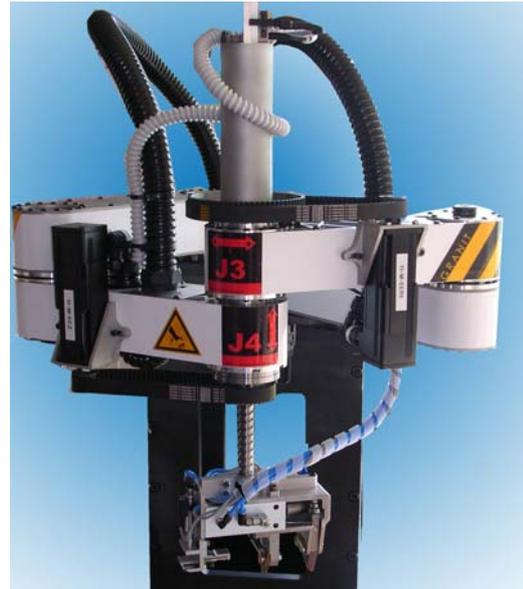
Fig. 3: The *GRANIT* parallel-kinematics robot
